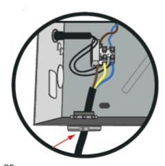
Through the side conduit knockout, which also directly connects AC power to the terminal block.
